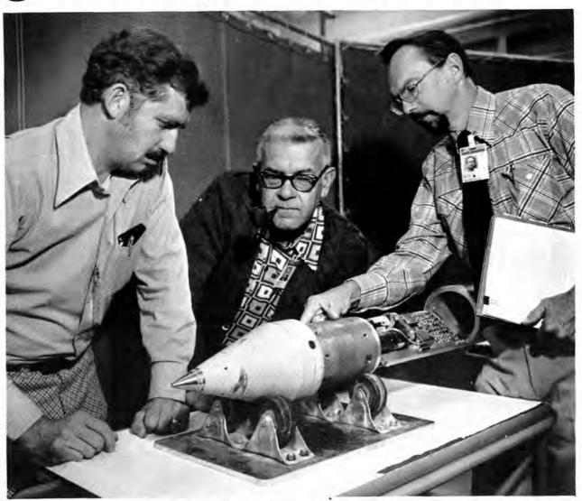
MAGMA TAP PROJECT includes development of air-dropped earth penetrator vehicles with instrumentation to take resistivity measurements and to sense subsurface heat for use in locating suitable magma sources. Twenty-nine penetrators were dropped in Hawaii recently to help with a University of Hawaii geothermal project. Another operation is planned with the University of Alaska. Wayne Young (5716), John Colp (5716) and Gien Brandvold (5710) discuss the program.
